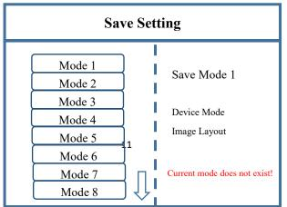
**Note:** Mode 1 is default startup data of device boot; it's suggested that the most common mode should be saved to Mode 1 and the device can save 32 kinds of mode at most.
