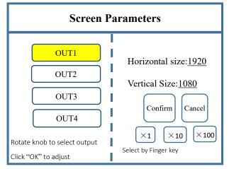
**Note:** Input according to corresponding transmitting card size of each output interface. For OUT1, its horizontal size is 1920 and vertical size 576; for OUT2, they are 1920 and 576 respectively; for OUT3, they are 1920 and 576; for OUT4, 1120 and 576.
