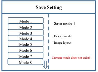
**Note:** Mode 1 is default startup data of device boot; it's suggested that the most common mode or that required by device boot should be saved to Mode 1.
