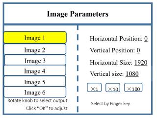
Step 5: Click "OK" and return to main menu interface; select "Clipped view" to enter into its setting interface to set size and position of each image.
