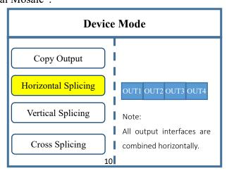
Note: since four transmitting cards are in a horizontal layout, horizontal mosaic is needed then.
