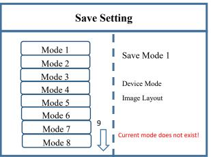
**Note:** Mode 1 is default startup data of device boot; it's suggested that the most common mode should be saved to Mode 1 and the device can save 32 kinds of modes at most.
