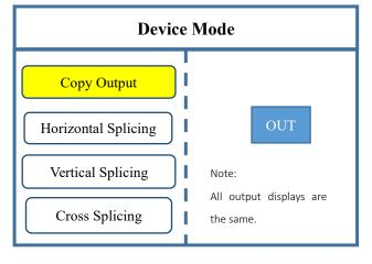
**Note:** Copy mode: all output contents are consistent; horizontal mosaic: content of all output are arranged horizontally; vertical mosaics: contend of all output are arranged vertically; cross mosaics: contend of all output are arranged in two rows and two columns.
