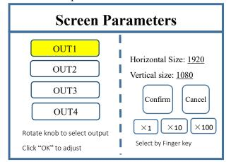
**Note:** Input according to corresponding transmitting card size of each output interface. For OUT1, its horizontal size is 1440 and vertical size 896; for OUT2, they are 1248 and 896 respectively; for OUT3, they are 1440 and 768; for OUT4, 1248 and 768.
