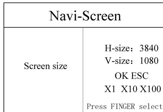
Set the screen parameters, set the horizontal size and vertical size as the actual number of LED screen resolution, click "OK" to complete the parameter settings
