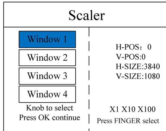
**Step 5:** Click "MENU" to return to the main menu interface, enter Menu - More - Common Functions - Partial Display, enter the part display setting interface, and set the size and position of the partial interception of each signal source.
