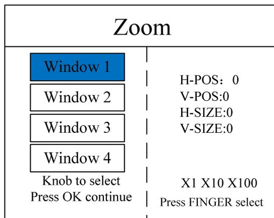
Note: Skip this step if the signal source picture needs to be completely displayed on the large screen; if you only need to capture a certain signal source in the multi-picture, you only need to set the picture of the signal source; horizontal size or vertical size A value of 0 indicates that no local interception is performed in this direction.
